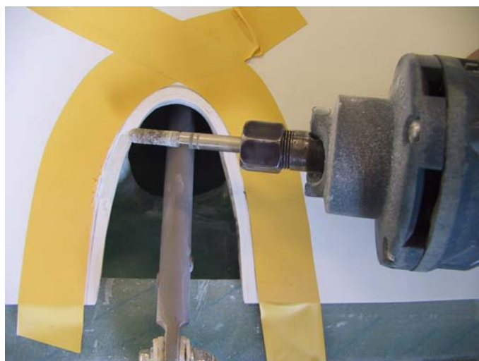
Step 8: - rasp of surface
